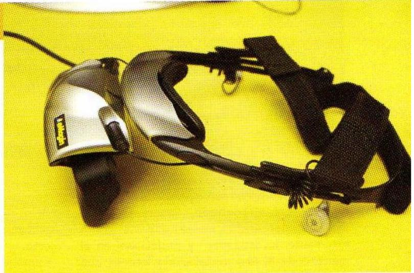
Figura 3. Lentes 3D (Head Mounted Display)
